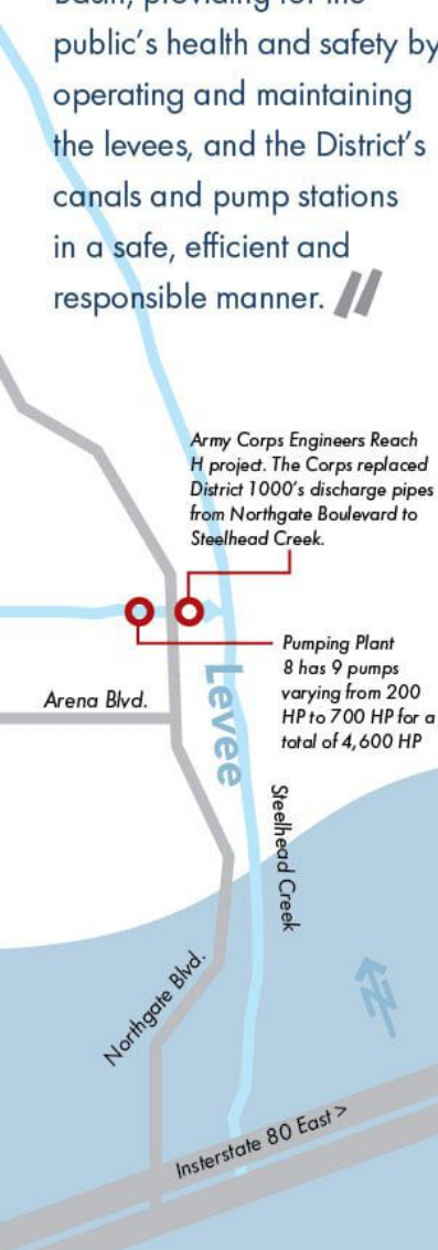
Pumping Plant 8 is called the C-1 drain. Which is fed from the north and south out of the east drainage canal west of pumping plant 8. Pumping Plant 8 has 9 pumps
